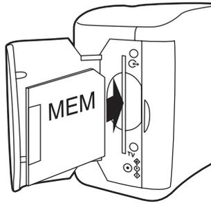
Make sure the card is pushed firmly into the slot.
